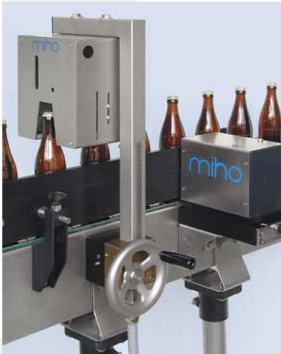
The miho **Newton HF** is the **HF Fill Level Control** in the miho **Newton** Fill Level Control Range. The fill level detection by means of high frequency technology is today the standard method, due to its **high level of reliability** and **economical price**.
